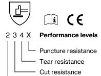
Pictogram and performance levels according to EN 388:2003 (highest performance level: 4/cut resistance: 5)
